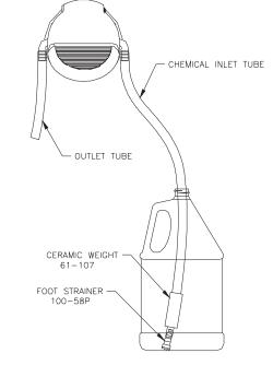
4. **SERVICING:** Flush with warm water to dissolve any dried fluid.
